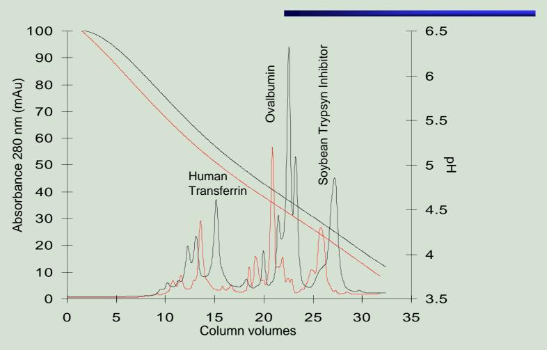
Analytical anionic plsep (black lines) and 8 times scale-up separation (red lines) of a mixture containing human transferrin, ovalbumin and soybean trypsyn inhibitor over the pH range 6.5-3.5. The pH gradient was developed over 30 column volumes (0.09 pH units per CV) on both analytical Mono Q HR 5/5 and the scale-up Mono Q HR 10/10 column at flow rates 1 ml/min and 4ml/min respectively. Proteins were purchased from Sigma and used without preliminary purification.
