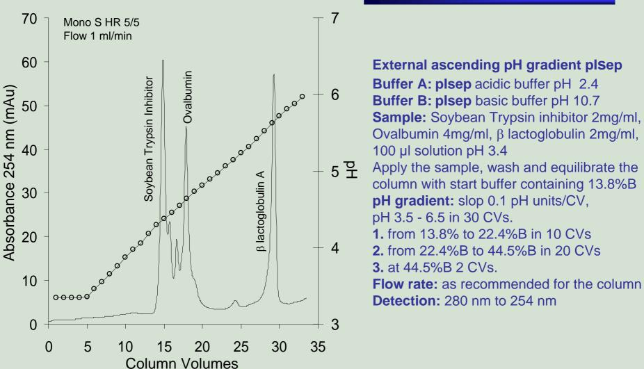
CryoBioPhysica resolution plsep test conducted on Mono S HR 5/5 high efficiency cation exchange column from GE Healthcare (formerly Amersham Biosciences)
