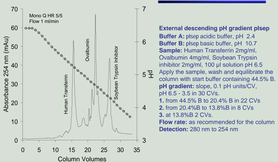
CryoBioPhysica resolution plsep test conducted on Mono Q HR 5/5 high efficiency anion exchange column from GE Healthcare (formerly Amersham Biosciences)
