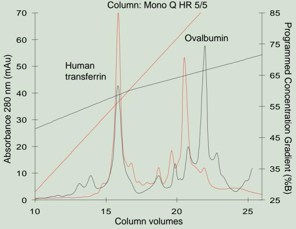
plsep versus anion exchange chromatography (AEX). Black lines: plsep fractionation of a mixture of human transferrin and ovalbumin: absorbance and profile of the external pH gradient, 0.098 pH units/column volume from pH 6 to pH 4; Red lines: AEX salt elution chromatography of the same proteins - absorbance and profile of the salt gradient, 9.4 mM NaCl/column volume from 0 to 0.3 M NaCl at pH 6.
