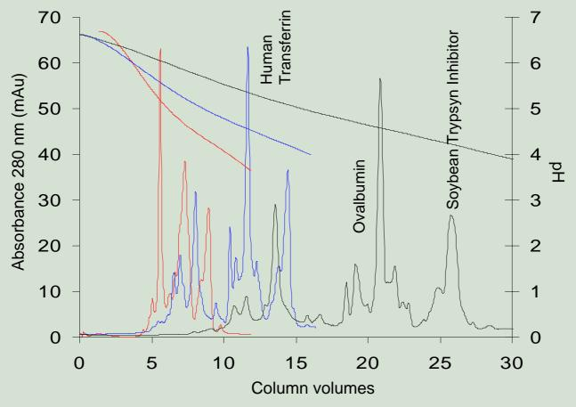
Anionic plsep separations of a mixture containing human transferrin, ovalbumin and soybean trypsyn inhibitor over the pH range 6.7-3.5. The effectiveness of the plsep fractionation is influenced by the slope of the pH gradient: red line – slope 0.25 pH units/CV; blue line – slope 0.15 pH units/CV and black line – slope 0.09 pH units/CV. Column: Mono Q HR 10/10, column volume 7.85ml, flow rate 4 ml/min. Proteins were purchased from Sigma and used without preliminary purification.
