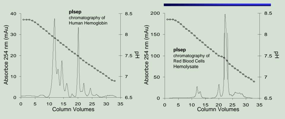
Buffer A: plsep acidic buffer pH 2.4, Buffer B: plsep basic buffer pH 10.7
