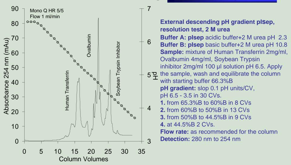
The chromatographer can resolve protein solubility issues by utilizing nonionic or zwitterionic detergents. Urea concentrations up to 8 M do not compromise the plSep separation resolution.
