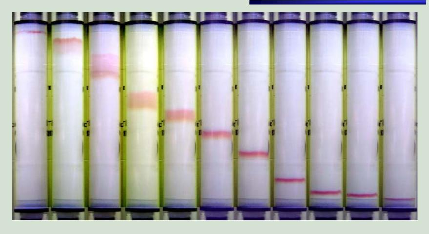
These photographs show the focusing effect observed during anionic **plsep** of horse myoglobin on Mono Q HR 5/5. Myoglobin molecules at the rear of the chromatographic band are at a pH lower than their pl and, as a consequence, are repelled from the anion exchanger and move faster than molecules at the front of the band where the pH is more alkaline than the pl of the protein. The result is progressive narrowing of the band and elution of myoglobin as a very sharp peak.
