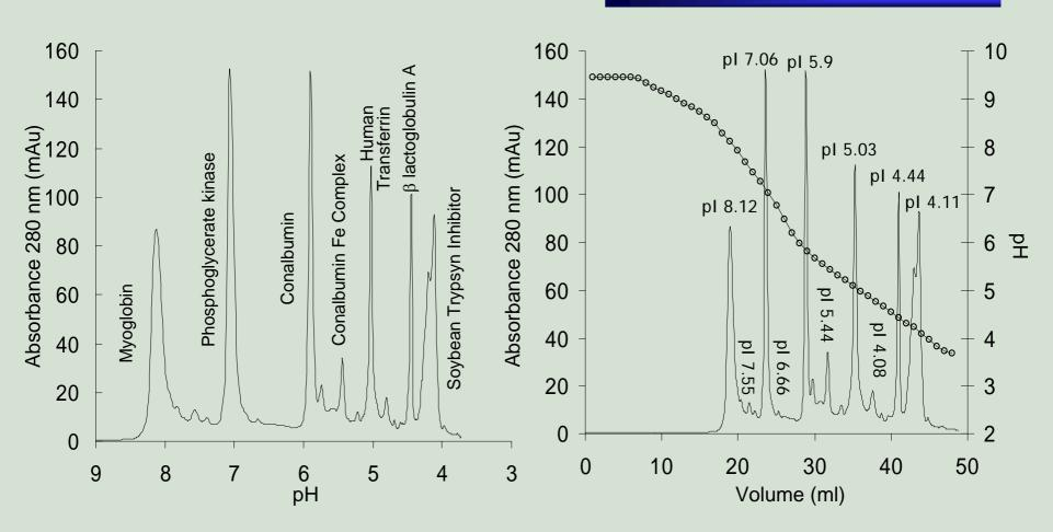
Separation of a complex mixture of proteins by external descending pH gradient plSep on a Mono Q HR 5/5 anion exchange column. The sample was loaded at pH 9.5 and eluted with an external pH gradient to pH 3.5. Despite the complexity of the sample, the closeness in pls for several species and the wide pH range necessary to separate all components, excellent resolution is achieved.
